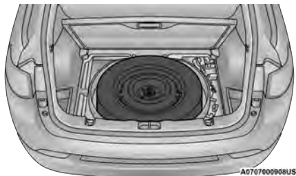
Damaged Tire Stowage
