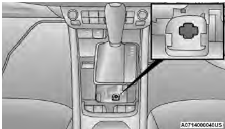
Gear Selector Override Access Hole
