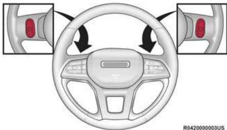
Remote Sound System Controls
