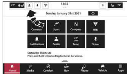
Uconnect 5/5 NAV With 10.1-inch Display Or 12-inch Display Changing The Upper Status Bar
