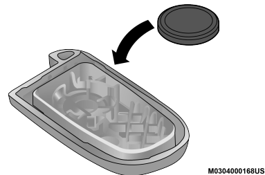
Key Fob Battery Replacement
