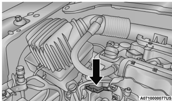
**Suitable Engine Ground (Example Engine Shown)**
