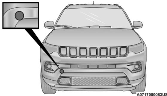
**Front Tow Eye Access Door**
