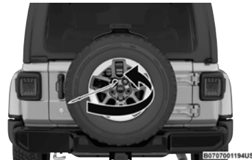
Removing The Spare Tire
