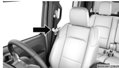
Pulling Out The Latch Plate
