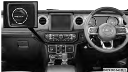
Front Power Outlet
