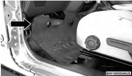
Front Carpet Pulled Away
