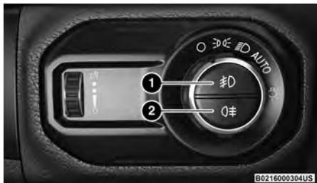
Fog Light Switch Location
