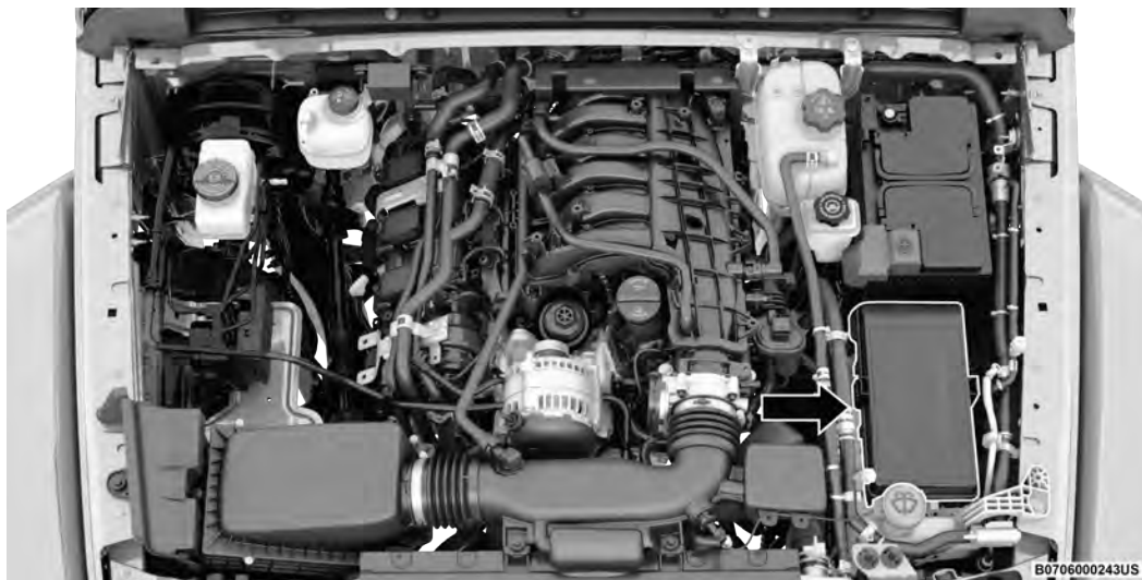
Power Distribution Center Location
