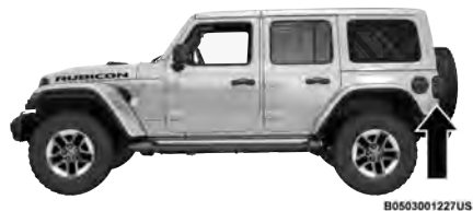
BSM Radar Location (Left Side Shown)
